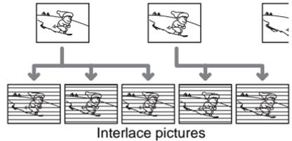
This player solves this problem by increasing the speed at which the frames are displayed, consecutively showing 3 identical frames followed by 2 identical frames in the time that it normally takes to show 2 consecutive frames. The end result is that the 24 frames per second are increased to 60 frames per second, which is the speed at which Progressive video signals are shown.
