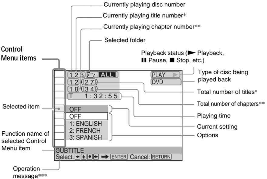
\* Displays the scene number for VIDEO CDs (PBC is on), track number for VIDEO CDs/Super Audio CDs/CDs, album number for DATA CDs.
