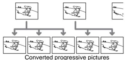
This not only allows film to be shown in a frame based format, it also increases the clarity and sharpness which is unique to Progressive format images.
