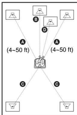
Be sure to change the value in the Setup Display each time you move the speakers. Start from the front speaker. The default adjustments are in parentheses.
