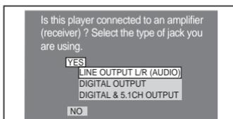
**11** Press  $\uparrow/\downarrow$  to select the type of jack (if any) you are using to connect to an amplifier (receiver), then press ENTER.
