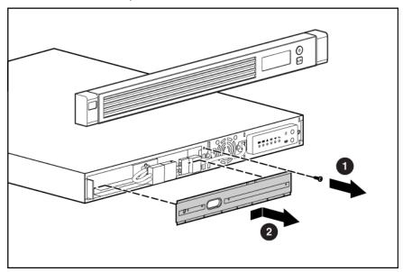
5. Remove the UPS battery modules.
