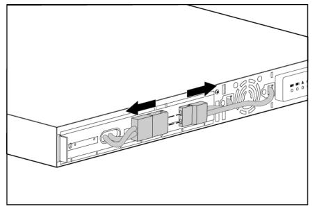
4. Remove the battery bracket.
