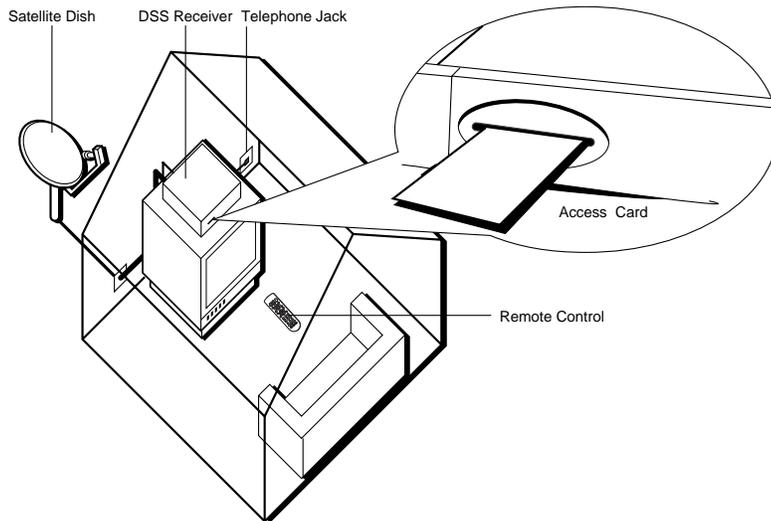
**DSS® Satellite Dish Antenna** Picks up the satellite's coded program information and relays it to your DSS® receiver. (Your satellite dish may be installed in different locations on or around your house. The satellite dish antenna must, however, be pointed in a southern direction toward the satellite.)
