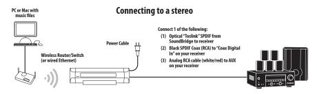
c. Connect to your stereo system using either coaxial SPDIF digital or optical SPDIF digital (the SoundBridge has connectors for both) — cables sold separately.
