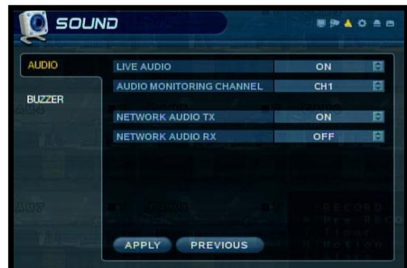
**NOTE:** Once the LIVE AUDIO Feature has been set to ON, the Remote Control can be used to select the Listen-In Audio Channel. Press the AUDIO SEL button on the Remote Control to switch between Channels 1~4. An Audio Icon will appear onscreen next to the current Live Audio Channel.
