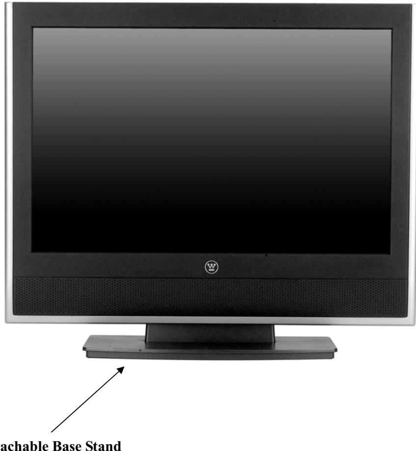
To detach the base stand, just press on the locking tabs on the bottom of the base stand and remove the base stand from the stand neck.
