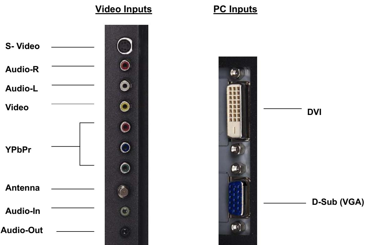
**Note:** The Audio-L and Audio-R (Audio L/R) inputs are shared between YPbPr, S-Video, and Video source input connectors.
