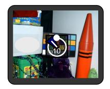
Note the timer icon in the center of the display. When the timer is on, and set to 10 seconds (for example), the front red LED begins blinking when the shutter button is pressed. It begins counting down with 8 seconds of slow blinking (with audio beeps if the sound is on) and 2 seconds of fast blinking (with audio beeps). After the picture is taken there is a 1 second audio beep and the red LED goes steady.
