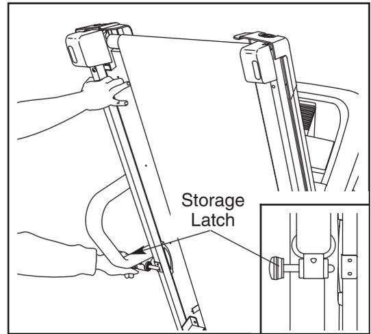
2. **Hold the metal frame firmly with both hands**, and lower it to the floor. **CAUTION: To decrease the possibility of injury, do not lower the frame by gripping only the plastic foot rails. Do not drop the frame to the floor. Make sure to bend your legs and keep your back straight.**
