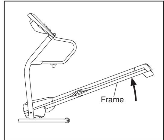
2. Move your right hand to the position shown and hold the treadmill firmly. Using your left hand, pull the latch knob to the left and hold it. Raise the frame until the catch passes the latch pin, and then slowly release the latch knob. **Make sure that the catch is held securely by the latch pin, as shown.**
