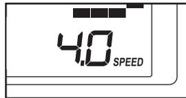
If one of the ten numbered buttons is pressed, the walking belt will gradually increase in speed until it reaches the selected speed setting. **Note: The console can display speed and distance in either miles or kilometers (see THE INFORMATION MODE/DEMO MODE on page 16). For simplicity, all instructions in this section refer to miles.**
