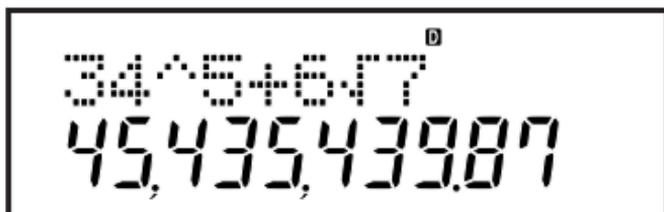
The two-line display makes it possible to view both the calculation formula and its result at the same time.
