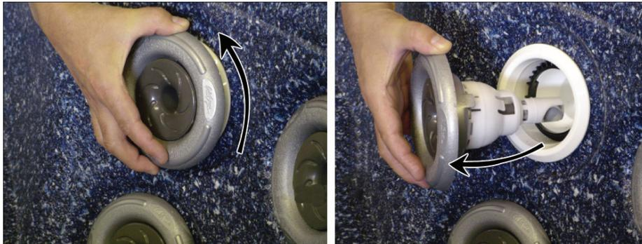
To replace jets, insert the jet in the jet well and push and rotate it clockwise until you feel it snap into position. When the jet face can be rotated freely, it is properly seated.
