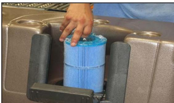
Unscrew the cartridge and remove it.
