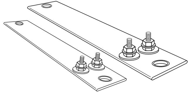
The Watlow mica strip heater is an economical and reliable source of heat for industrial equipment. A mere 15 mils (0.4 mm) thick mica insulator on both sides of the resistance element provides complete electrical insulation and offers little resistance to efficient heat flow. Plus mica withstands high voltage spikes, resists moisture and is inert to most chemicals. UL® component recognition is available for applications to 900°F (480°C) sheath temperature, file number E52951.
