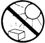
Use and store the equalizer/booster only in normal temperature environments. Temperature extremes can shorten the life of electronic devices and distort or melt plastic parts.
