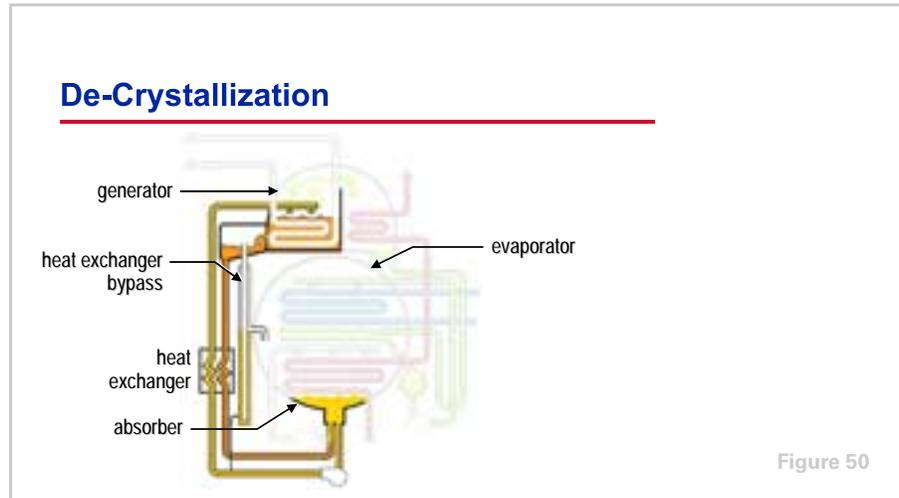
As a second line of defense, most absorption water chillers include devices that allow the chiller to recover in the event that crystallization does occur. Some of these devices simply sense impending crystallization, put the chiller through a dilution cycle, and shut the chiller down. Other devices keep the chiller operating while regaining control of the solution temperature and concentration.
