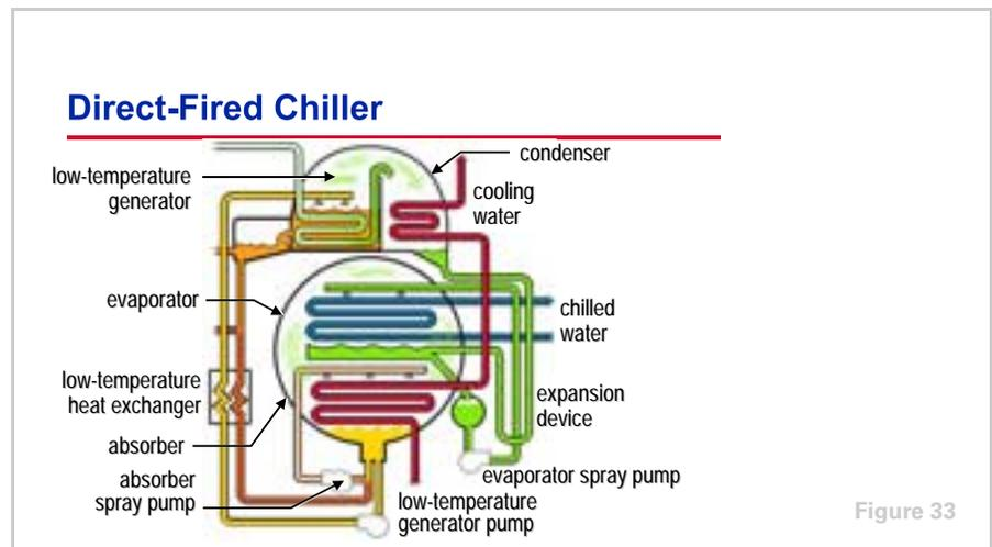
Next, the refrigerant travels through the condenser, expansion device, evaporator, and absorber in a manner similar to refrigerant travel in the indirect-fired double-effect absorption chiller.
