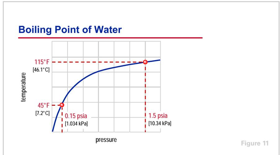
At a given pressure, the temperature at which a liquid will boil into a vapor is the same temperature at which the vapor will condense back into a liquid. This curve illustrates the pressures and corresponding temperatures at which water (the refrigerant) boils and condenses.
