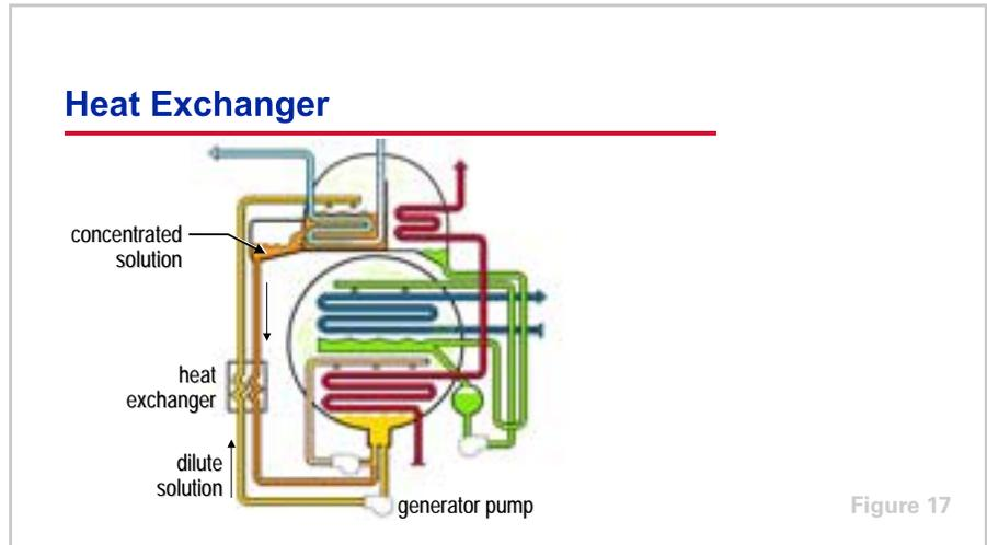
As the lithium bromide solution absorbs the refrigerant, it becomes diluted and has less ability to absorb water vapor. To complete the cycle and sustain operation, the absorbent solution must be reconcentrated. Consequently, the **generator pump** continuously returns the dilute solution to the generator to again separate the refrigerant vapor from the solution and reconcentrate the solution, thus repeating the cycle.
