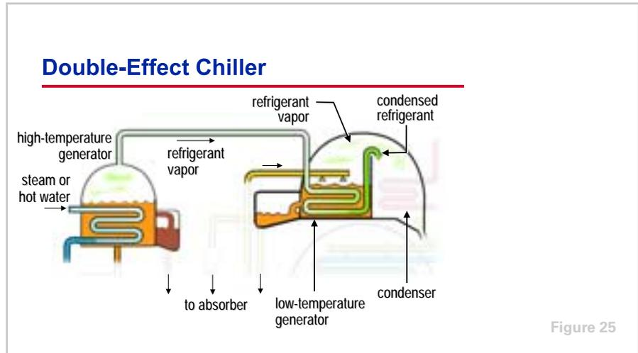
In the **high-temperature generator**, very high temperature steam or hot water flows through tubes that are immersed in an absorbent solution that is at an intermediate concentration. The solution absorbs heat from the warmer steam or water, causing the refrigerant to boil and separate from the absorbent solution. As the refrigerant boils away, the absorbent solution becomes concentrated and returns to the absorber.
