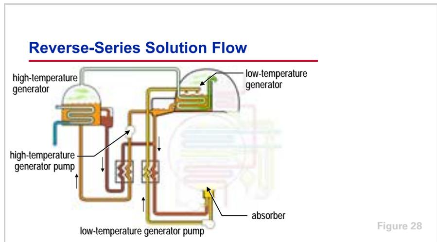
All double-effect absorption chillers are constructed from the same basic components: high-temperature generator, low-temperature generator, condenser, evaporator, absorber, two solution heat exchangers, and several pumps. There are, however, three common methods in which the solution can be circulated through the chiller: series, parallel, and reverse-series. The double-effect chiller used in the previous example employs the reverse-series flow cycle.
