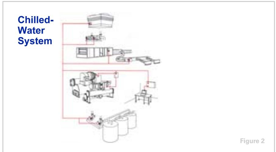
Water chillers are used in a variety of air conditioning and process cooling applications. They are used to make cold water that can be transported throughout a facility using pumps and pipes. This cold water can be passed through the tubes of coils to cool the air in an air conditioning application, or it can provide cooling for a manufacturing or industrial process.
