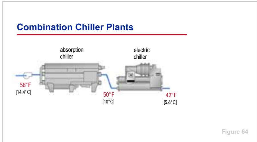
The second beneficial operating characteristic is that an absorption chiller works more efficiently and produces more cooling with increased leaving-chilled-water temperatures.
