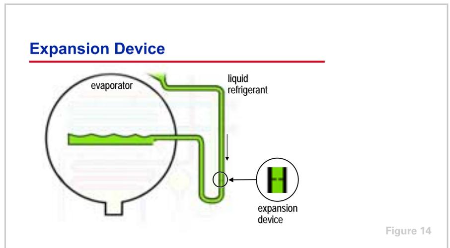
From the condenser, the liquid refrigerant flows through an **expansion device** into the evaporator. The expansion device is used to maintain the pressure difference between the high-pressure (condenser) and low-pressure (evaporator) sides of the refrigeration system. In this example, the expansion device is a throttling pipe, which is a long section of pipe with an orifice restriction in it. It creates a liquid seal that separates the high-pressure and low-pressure sides of the cycle.
