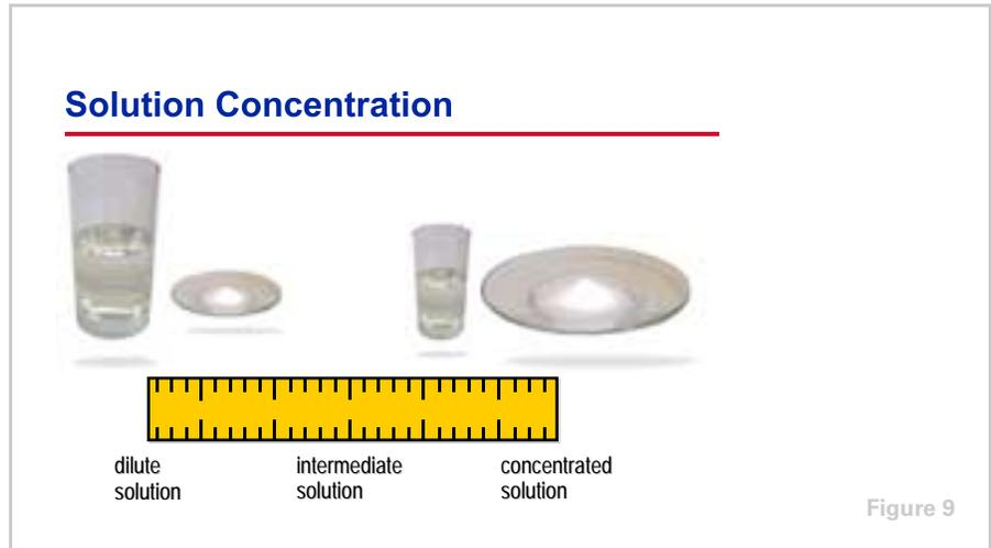
These two fluids, the refrigerant and the absorbent, are mixed inside the chiller in various concentrations. The term **dilute solution** refers to a mixture that has a relatively high refrigerant content and low absorbent content. A **concentrated solution** has a relatively low refrigerant content and high absorbent content. An **intermediate solution** is a mixture of dilute and concentrated solutions.
