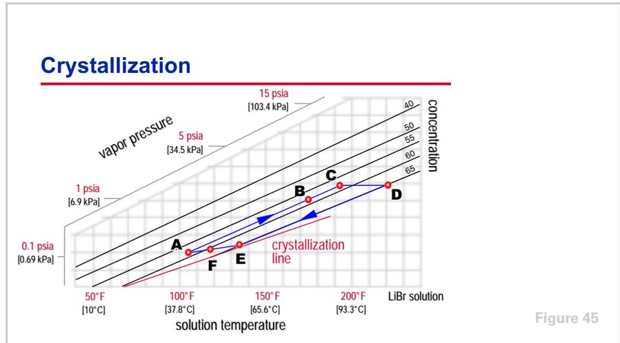
By plotting the single-effect absorption refrigeration cycle on the equilibrium chart, it is apparent that crystallization is most likely to occur in the heat exchanger. At this particular condition, the 65% concentrated solution (**D**) is cooled to 135°F [57.2°C] (**E**) as it passes through the heat exchanger. As noted previously, the saturation temperature of 65% solution is 123°F [50.6°C] so there is no danger of crystallization.
