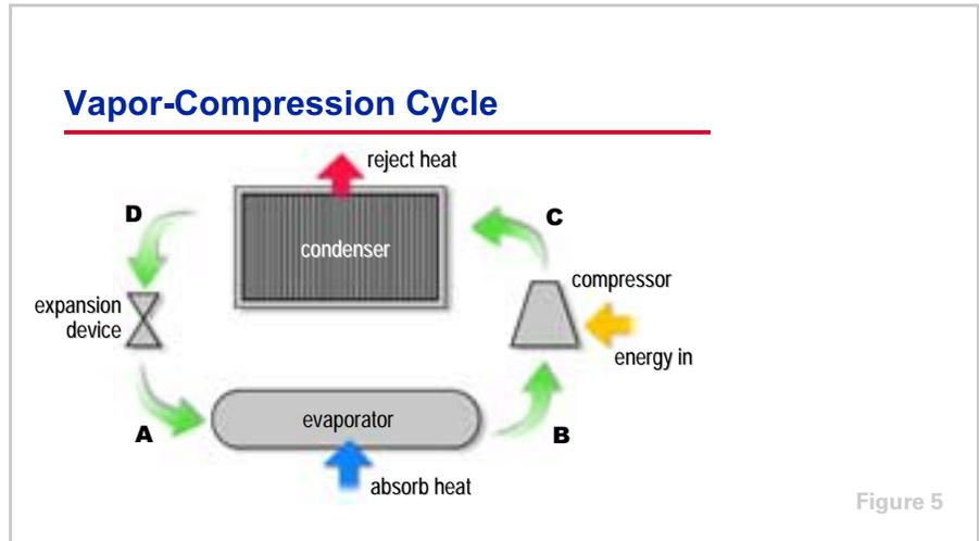
In the vapor-compression refrigeration cycle, refrigerant enters the evaporator in the form of a cool, low-pressure mixture of liquid and vapor (**A**). Heat is transferred from the relatively warm air or water to the refrigerant, causing the liquid refrigerant to boil. The resulting vapor (**B**) is then pumped from the evaporator by the compressor, which increases the pressure and temperature of the refrigerant vapor.
