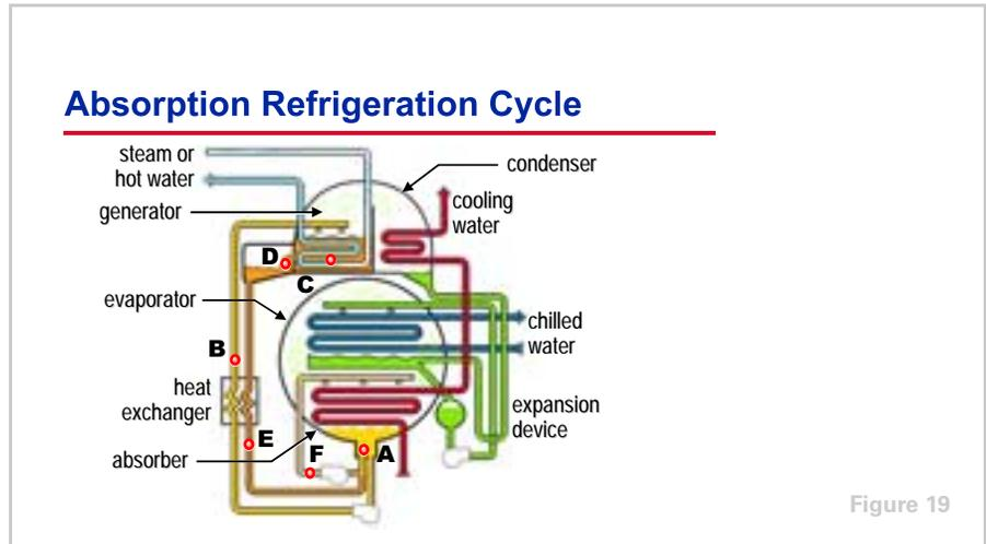
A diagram of a typical absorption refrigeration cycle can be superimposed on this equilibrium chart to demonstrate the function of each component in the system.
