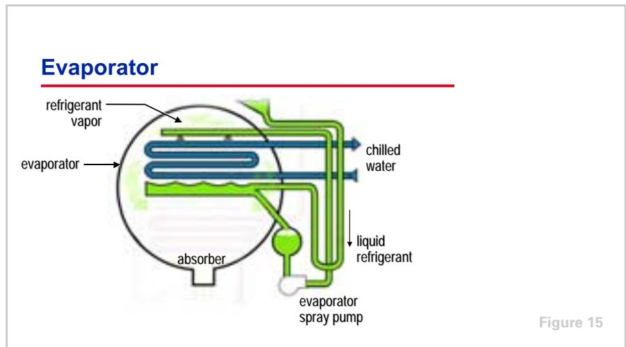
Inside the **evaporator**, relatively warm return water from the chilled-water system flows through the tubes. An **evaporator pump** draws the liquid refrigerant from the bottom of the evaporator and continuously circulates it to be sprayed over the tube surfaces. This maximizes heat transfer.
