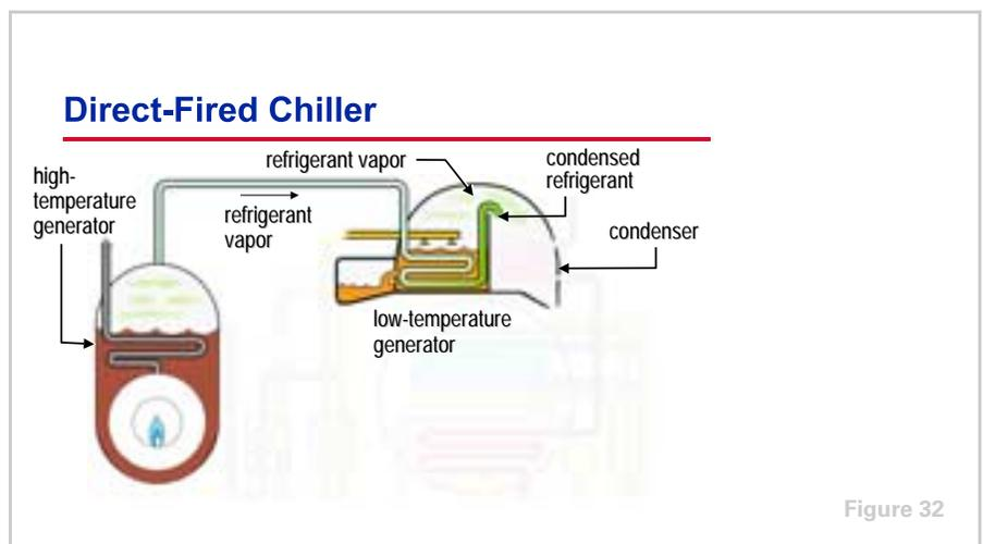
The example direct-fired chiller shown here employs the reverse-series flow cycle. In the **high-temperature generator**, the intermediate solution absorbs heat that is generated by the combustion process. Similar to the indirect-fired, double-effect chiller, this transfer of heat causes the refrigerant to boil and
