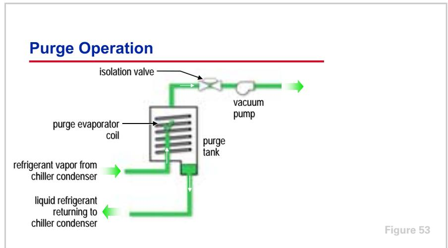
This example purge system consists of a purge tank, a small refrigeration system, a pump-out system, and controls. The purge's refrigeration system includes: a small compressor, an air-cooled condensing coil, an expansion valve, and an evaporator coil located inside of the purge tank.
