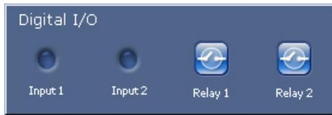
The alarm icons **Input 1** and **Input 2** are for information purposes and indicate the status of an alarm input: When an alarm is triggered, the corresponding icon lights up blue. The camera's configuration determines whether the alarm is displayed, as well as additional details (see *Section 5.14 Advanced Mode: LIVEPAGE Functions, page 38*).
