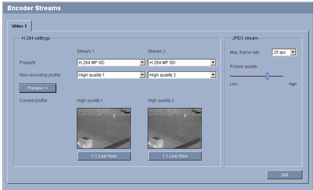
The VOT-320 simultaneously generates two H.264 data streams (Dual Streaming); you can select the relevant property for these here and connect them to an encoder profile, for example one for transmissions to the Internet and one for LAN connections.
