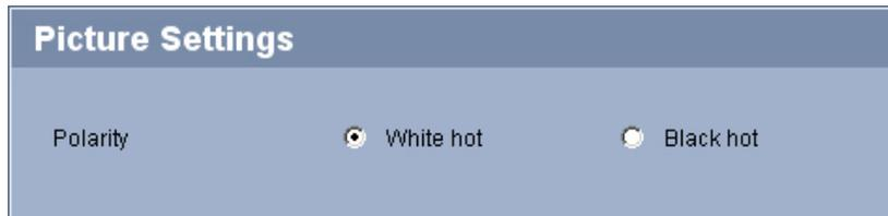
You can set the polarity of the thermal image of the camera to suit your requirements. The current video image is displayed in the small window next to the radio buttons as confirmation. Your changes are effective immediately.
