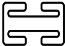
Remove locking clip when not using child restraint. Store under it's tab on the rear of seat.
