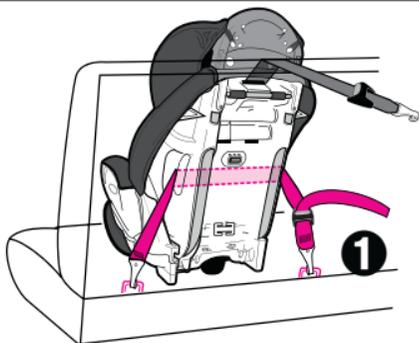
1. Unhook **LATCH** from storage bars on the sides of the seat. For ease of installation, extend **LATCH** to its maximum length.
