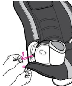
9. Pull the seat pad out of the way to reveal the red buttons as shown in the seating area ⑨. Slide the buttons to release the back support from the base and lower it into a flat position. Hold the back support to avoid it from falling back and hitting something.
