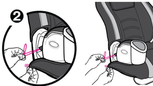
3. Pull the seat pad out of the way to reveal red buttons as shown in ③. Slide the buttons to release the back support from the base and lower it into a flat position.
