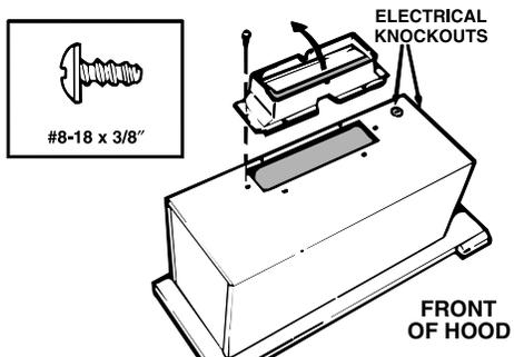
Use two (2) screws (provided) to attach the connector to the housing. The damper flap should open in the direction indicated by the arrow.
