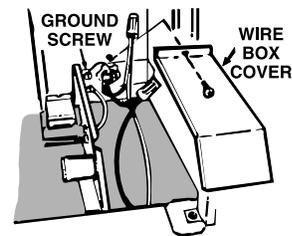
Remove the wire box cover. Attach the power cable to the hood using the proper connector. Connect black to black, white to white and green or bare wire to ground screw. Replace the wire box cover.
