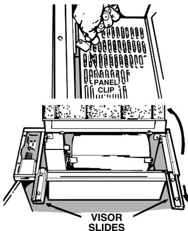
Pull the visor slides out. Rotate the panel clips and swing the panel open.
