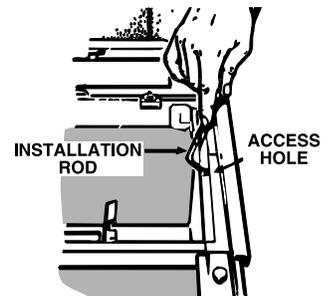
Insert the bent end of the installation rod into the access hole in the housing.
