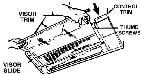
Slide the glass into the visor slides, above each visor clamp (see the illustration in step 14). Align the visor trim and tighten the thumb screws to secure the glass.
