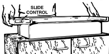
Carefully lower the housing into the cabinet opening with the slide control to the front
