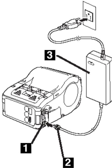
2. Connect the AC adapter to the wall outlet and turn on the power.
