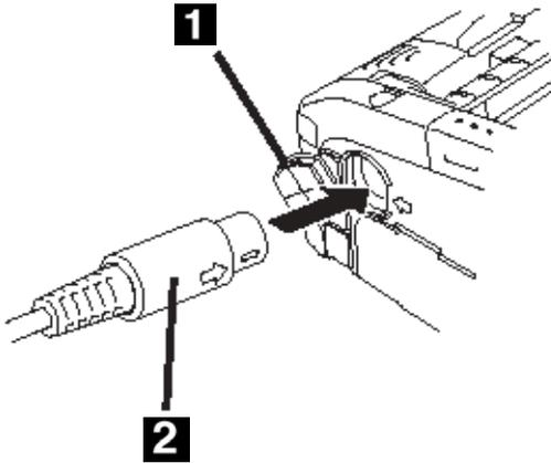
2. Plug one end of the RS-232C cable (2) firmly into the port. Make sure that the arrow mark on the connector of the RS-232C cable matches with the arrow mark by the side of the printer's port.
