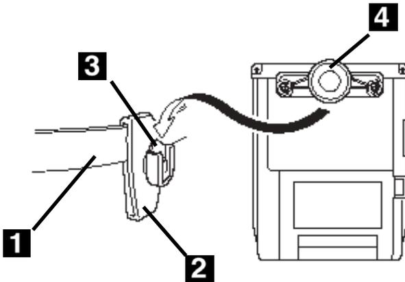
1. Thread your belt (1) through the belt holder (2), with the open end (3) of the clip mechanism up..
