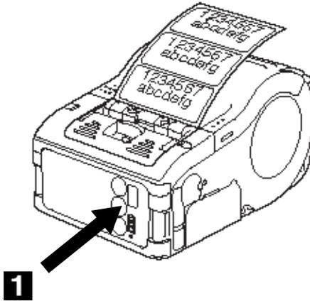
2. Press the FEED button (1) to feed a label.
