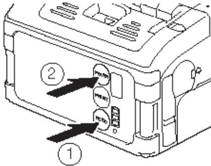
*The printer powers up in the test mode.*
