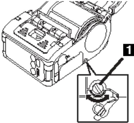
5. Turn the label roll lightly by hand and confirm that it rotates smoothly. Otherwise, paper may not be fed correctly during operation.
