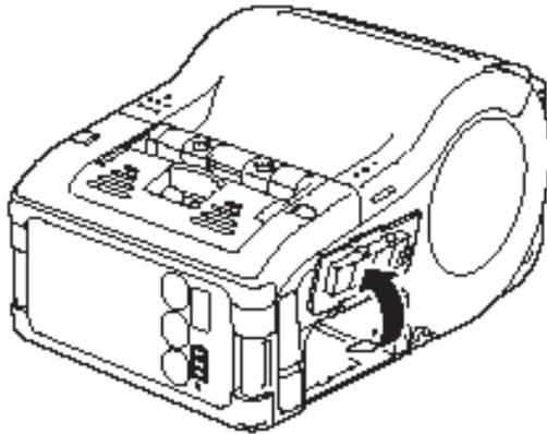
3. Push aside the gray latch (1) in the compartment, grasp the tab (2) on the top of the battery pack (3) and pull it out.
