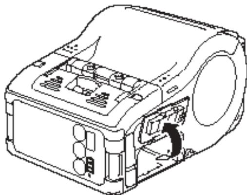
3. Align the battery pack so that its metal terminals (1) are facing the printer and the tab (2) on the battery is up, then insert the battery until it snaps in place.
