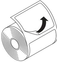
4. Place the label roll in the printer. Make sure it is placed with the leading edge (1) feeding up from the bottom of the roll and not down from the top.
