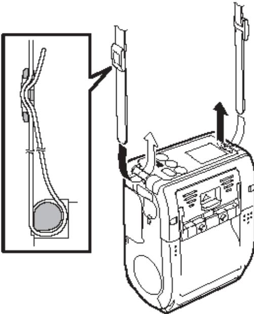
1. Feed one end of the shoulder strap through one of the channels at either side of the front of the printer.
