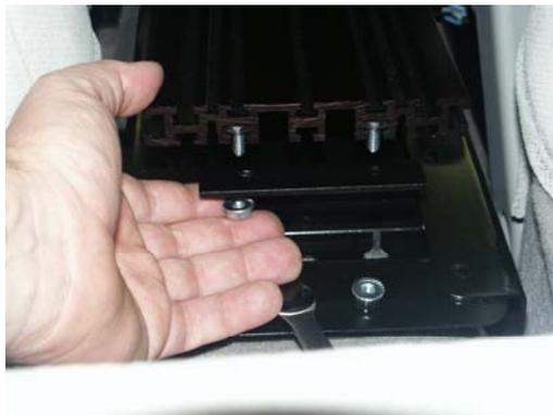
Attach rear extension bracket to 12" portion of extrusion using (2) 1/4-20 x 3/4" bolts and serrated nut
