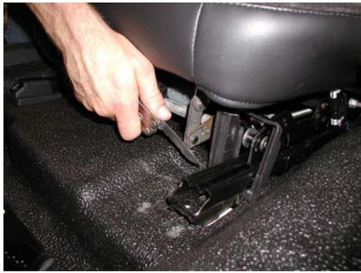
Cut floor mat, next to the seat rail to allow Under seat support bracket to slide under seat rail
