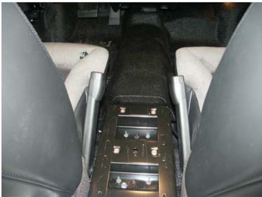
View of partial OEM console removed
