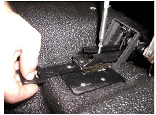
Slide guide brackets into seat rail and loosely attach #10 x 3/4" Phillips pan head machine screws
