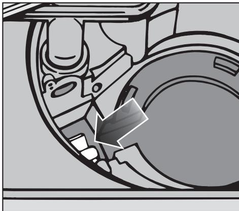
The drain pump is located beneath the non-return valve (arrow).
