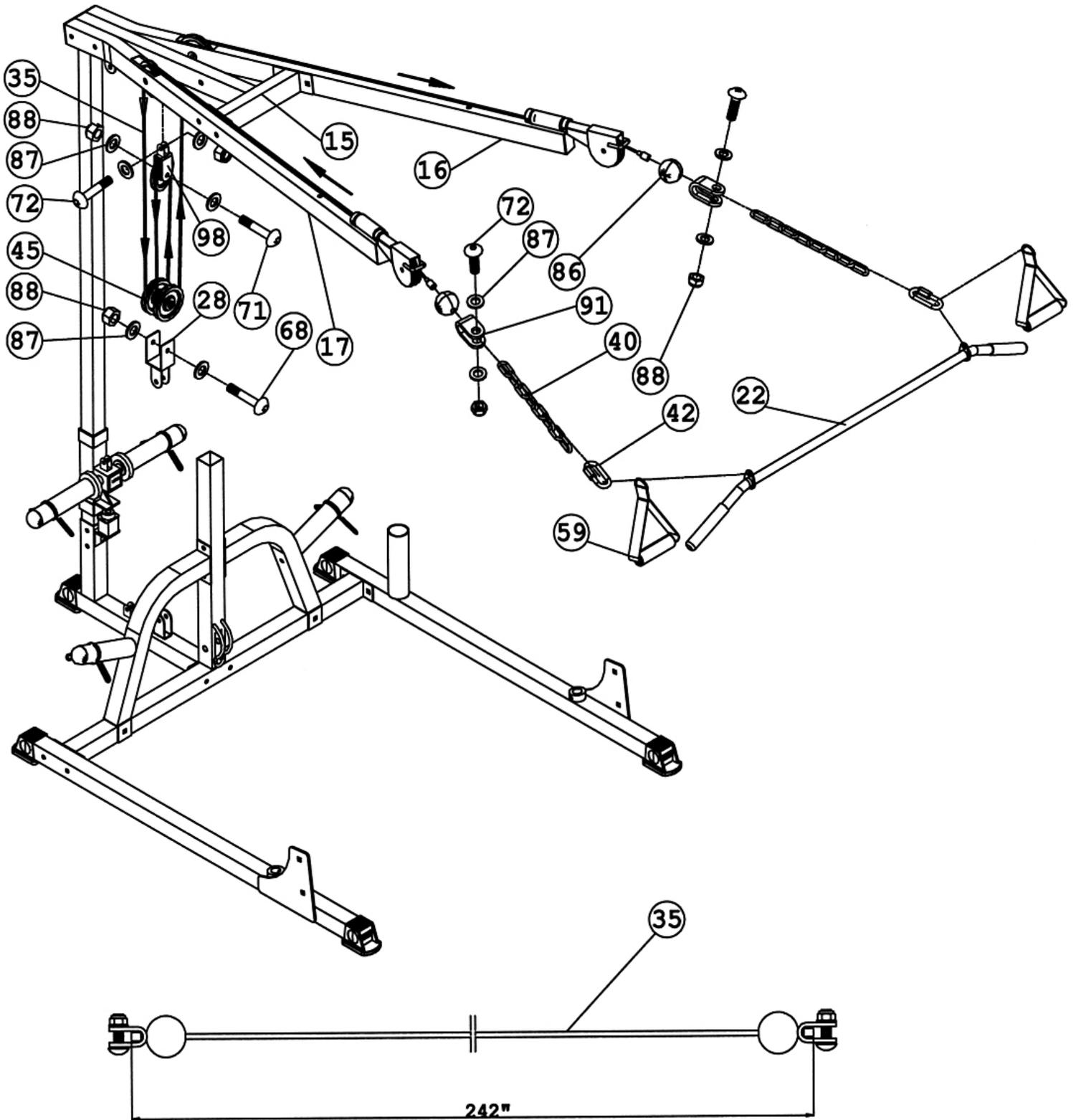
**STEP 7 (See Diagram 7 & Cable Loop Diagram)**
