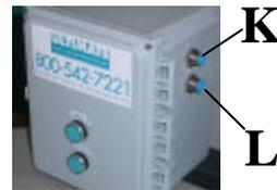
Connect air line from compressor      To      Left side of Control box
