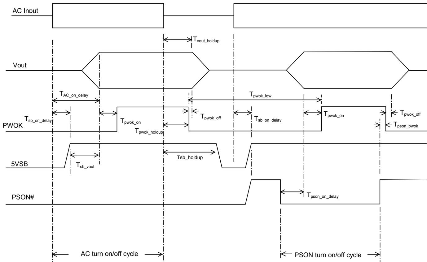
Figure 3: Turn On/Off Timing (Single Power Supply)
