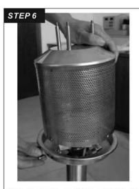
6-1. Put the emitter screen on the burner.
