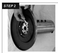
2-1. Use 4pcs M6X15mm bolts to fix the tank housing to the base & cast iron.
