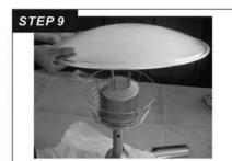
9-1. Put the reflector through the pins and on the washers.
