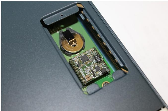
9. Double-check the new modem placement to make sure it is done properly.
