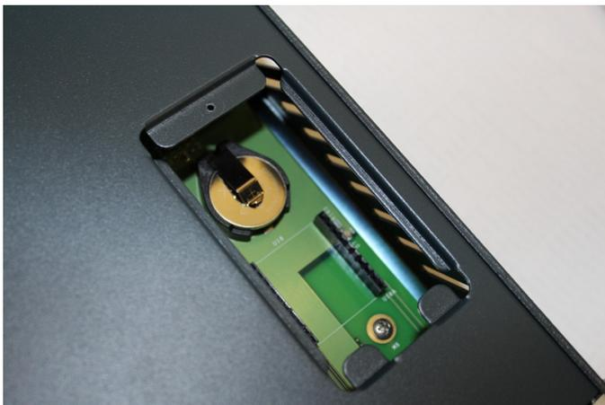
8. Re-install the modem with correct orientation.
