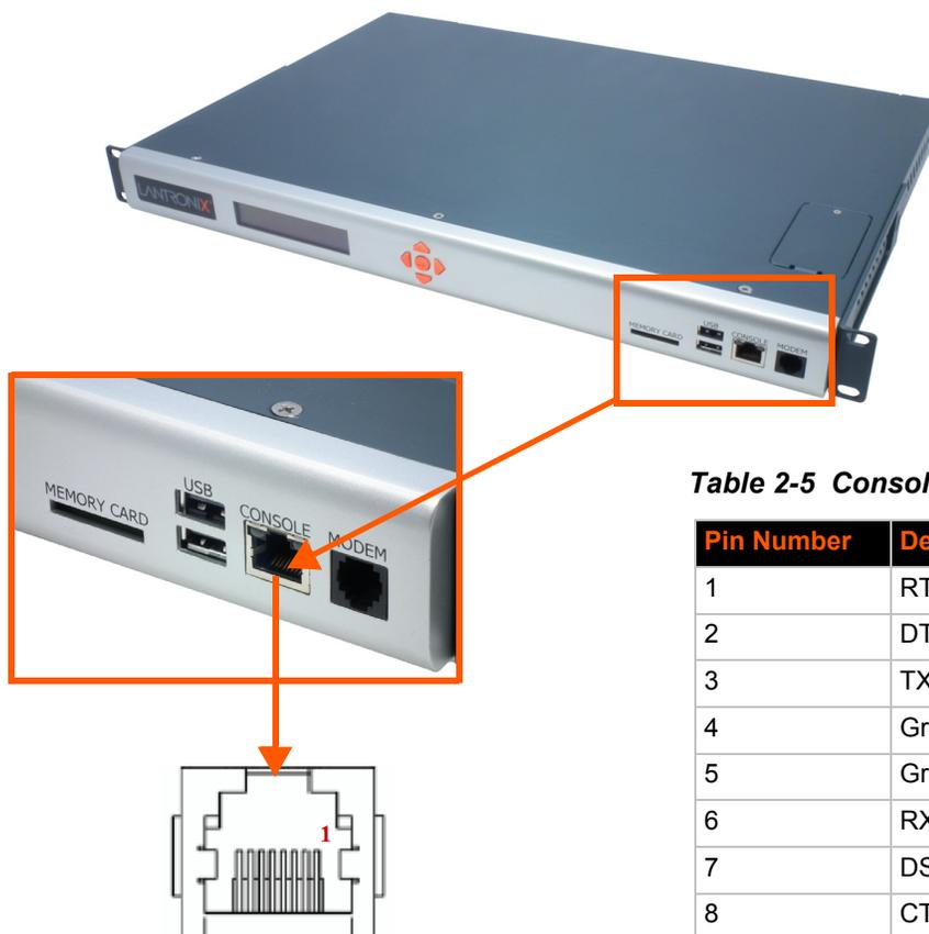
Table 2-5 Console (DTE) Port Pinout
