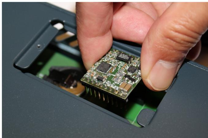
6. Install the new modem with correct orientation.
