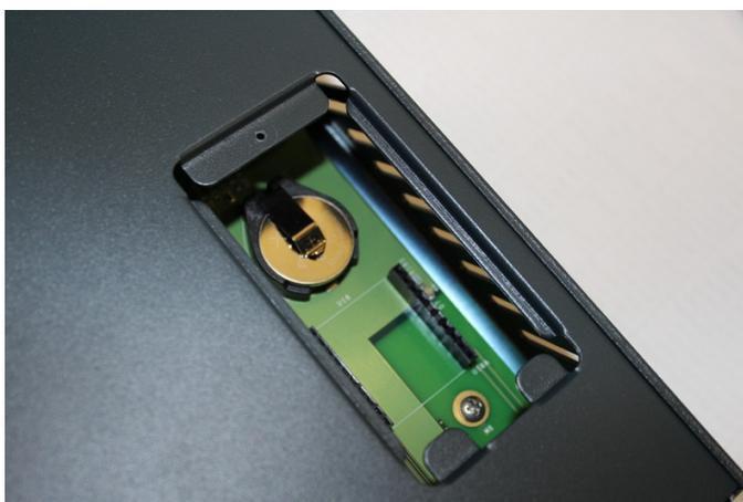
8. Press the modem down to make sure it sits down all the way in the socket.
