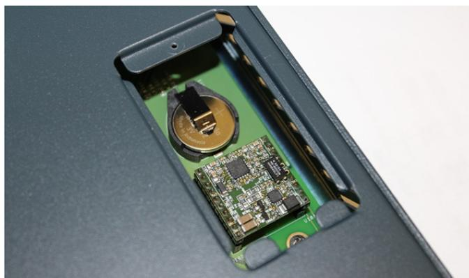
9. Double-check the battery and modem placements to make sure they are done properly.
