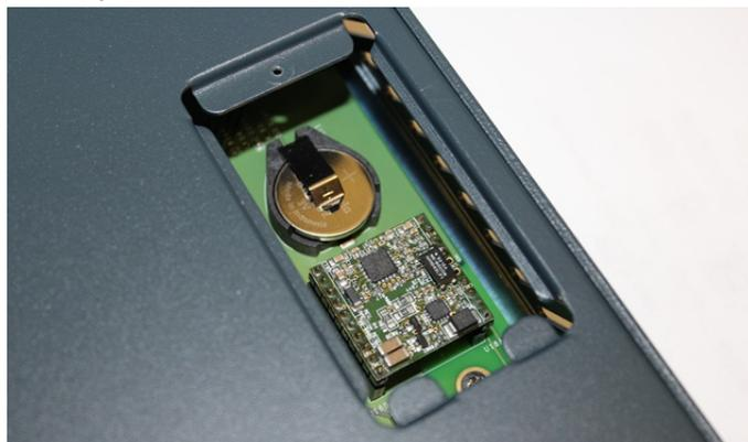
5. If there is a modem, carefully lift the modem out of its socket.
