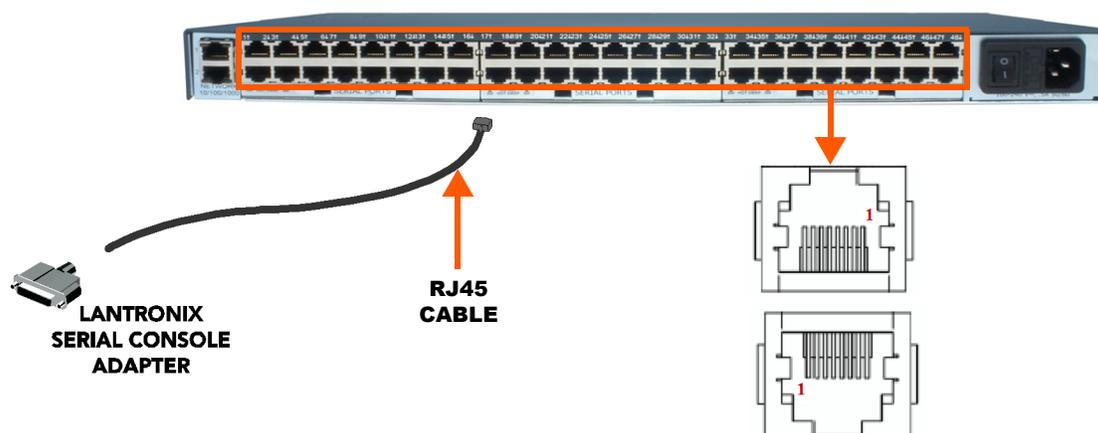
3. Connect the adapter to the serial console port on the serial device as shown in [Figure 3-3](#).
