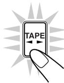
When the tape plays to the end, the deck automatically stops if the Reverse Mode is not on. (See “To play both sides repeatedly — Reverse Mode.”)
