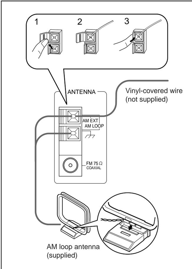
**1 Connect the AM loop antenna to the AM LOOP terminals as illustrated.**
