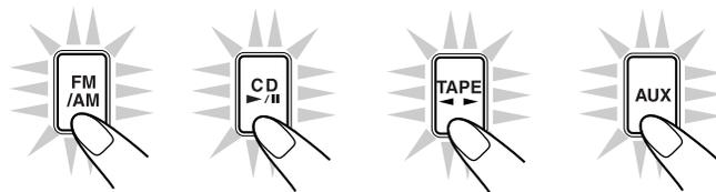
When you press the play button for a particular source (FM/AM, CD >||, AUX, and TAPE <>), the unit turns on, and the Powered Rolling Panel opens automatically (and the unit starts playing the source if it is ready — COMPU PLAY CONTROL).
