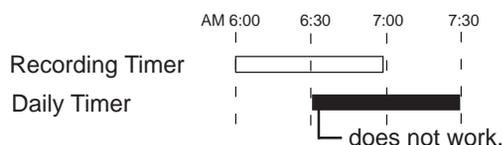
If Recording Timer is set to come on while Sleep Timer is operating, Sleep Timer will not work (the SLEEP indicator does not go off).
