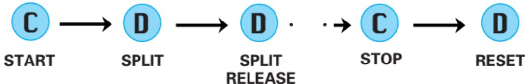
\* Measurement and release of split time can be repeated by pressing **Button D**.
