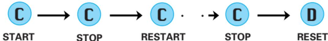
\* Restart and stop of stopwatch can be repeated by pressing **Button C**.
