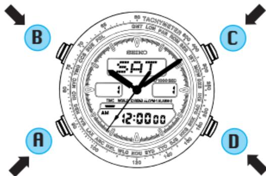
Press and hold the four buttons at the same time for 2 to 3 seconds.
