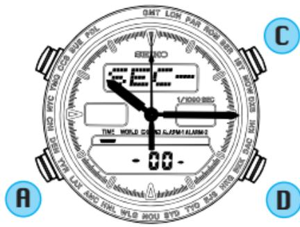
**C** Press to select the digits (flashing) to be adjusted in the following order (See \*1 on page 24):
