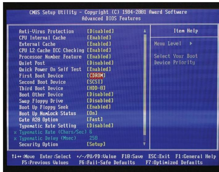
7. Press the Enter key. The First Boot Device dialog box opens. Scroll down to CDROM, and then press the Enter key to make the CD-ROM the first boot device.
