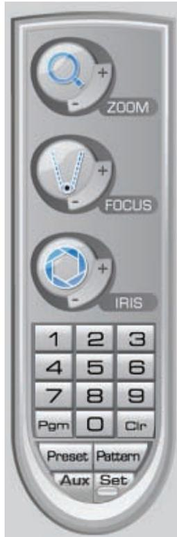
**Figure 32.** PTZ Keypad with Camera Lens Controls
