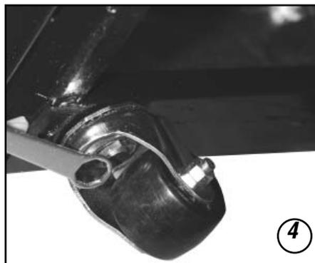
Tighten castor in position with castor wrench.
