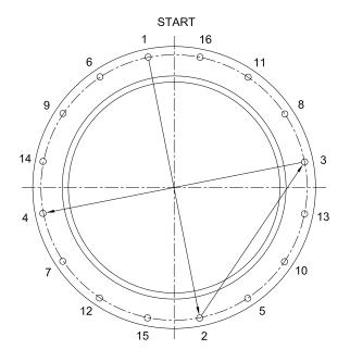
WARNING: It is extremely important to follow a proper tightening sequence. If not followed, the flanges can become cocked and a leak will result. When tightening flanges with spiral wound gaskets, if cocking occurs, the result can be deformation and non-repairable damage to the gaskets in addition to a resultant leak. Any gasket leak can result in potential injury to adjacent personnel.
