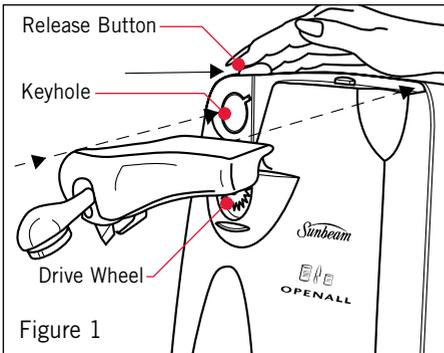
The Cutting Assembly fits into the keyhole opening at the top of the Open All™ can opener, above the Drive Wheel. Slide the Release Button to the right as the Cutting Assembly is inserted, it will “click” into position, with the release button returning to its original position.
