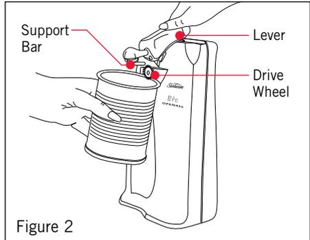
4. Firmly press the Lever down. This action will bring the blade down and pierce the lid of the can and start operating the motor to turn the can. Ensure the Magnetic Lid Holder is in contact with the lid of the can. (See figure 3.)
