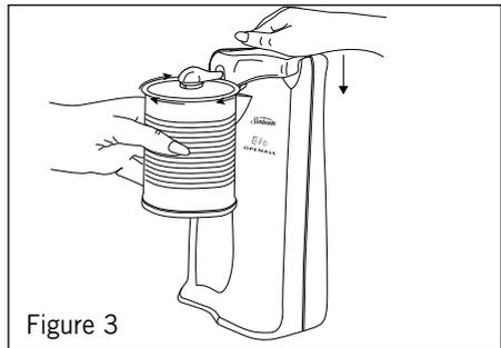
5. When the can begins to turn, it is no longer necessary to hold down the Lever.
