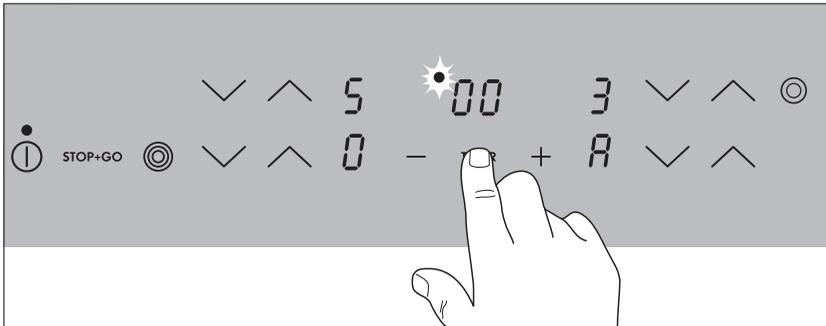
By touching the timer sensor panel once the first active cooking zone is selected in a clockwise direction, and the corresponding control lamp will flash rapidly. Hereby the (e.g.) left rear control lamp corresponds to the left rear cooking zone. **00** will appear in the timer display.
