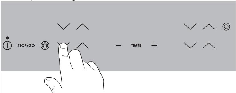
The displays will become dark, and the child safety device is switched off. The appliance will switch itself off automatically after a few seconds.
