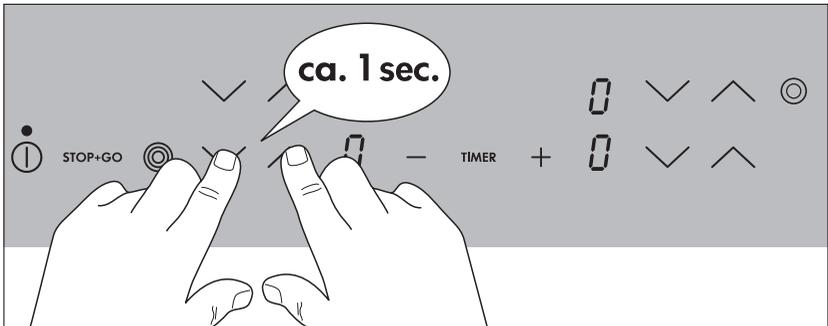
An acoustic signal will sound as confirmation. The child safety device has been overridden until the appliance is switched off, and the cooking surface can be used as normal.
