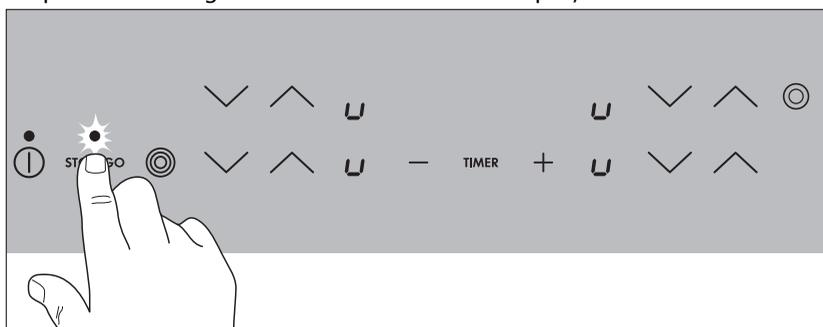
When the "Stop+Go" sensor panel is actuated again, the cooking settings that were previously selected are reset and the control light goes out.
