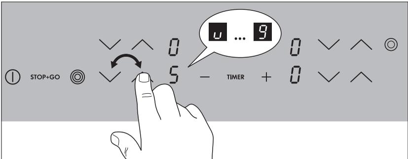
Raise the heat setting using the heat setting selector sensor panel
