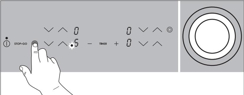
This will switch the setting to the centre heating ring. The lower control lamp will illuminate.
