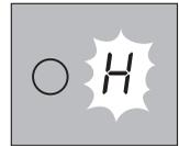
Even after the cooking zone has been switched off, the residual heat indicator only goes out when the cooking zone is cold.
