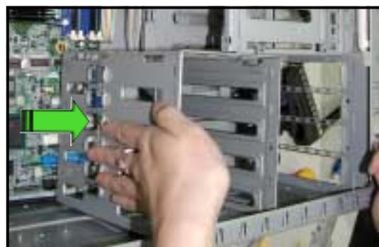
3. Make sure that the drive cage is fits snugly to the bay as shown. The drive cage is properly installed when it is parallel to the front panel, and the screw hole matches the hole of the first drive cage.
