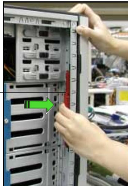
2. Pull and swing the left edge of the front panel outward.
