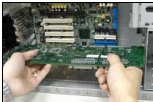
4. Push the card connector into the PCI slot until it is securely seated.
