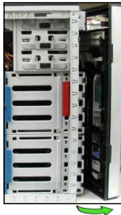
3. Unhook the hinge-like tabs from the holes on the right side of the front panel to completely detach the front panel assembly from the chassis.
