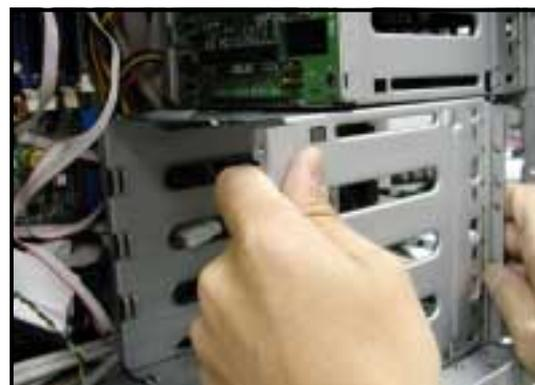
3. Make sure that the cage lock tab snaps to the bottom of the first drive cage. When properly installed, the cage should align with the first drive cage.
