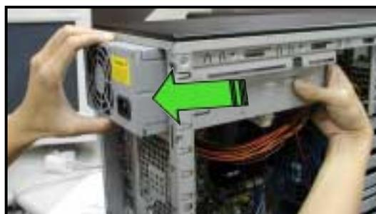
To install a power supply module:
