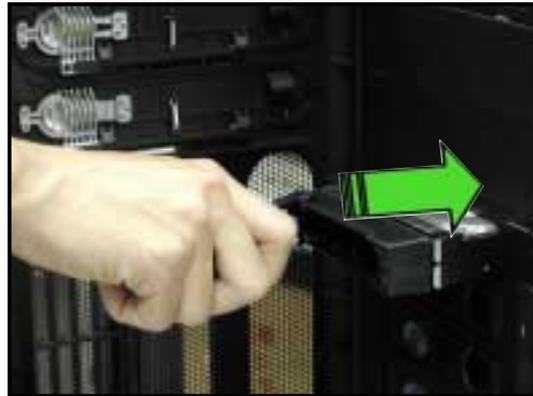
7. Push the tray lever until it clicks, and secures the drive tray in place. The drive tray is correctly placed when its front edge aligns with the bay edge.
