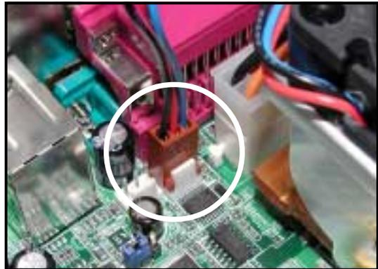
5. Repeat steps 1 to 2 to install the heatsink and fan assembly for the second CPU, then connect the fan cable to the fan connector labeled CPUFAN2.
