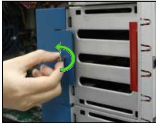
2. Hold the outer side of the fan cage, then pull sideways to release it from the chassis.
