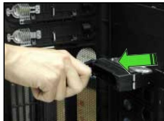
4. An empty drive tray requires a metal bracket for support. Use a Phillips (cross) screwdriver to remove the bracket if you wish to install a hard disk in the drive tray.
