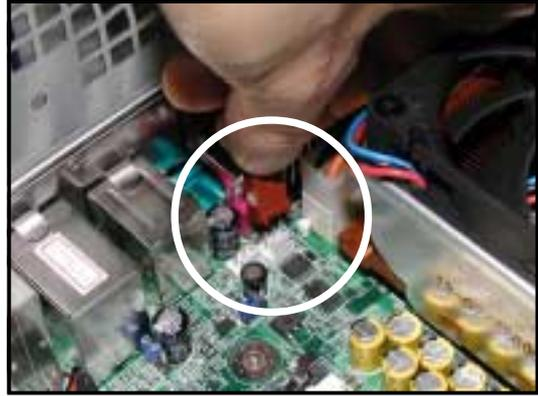
4. Make sure that the heatsink and fan assembly is stable in place and the fan power cable plug is properly connected.
