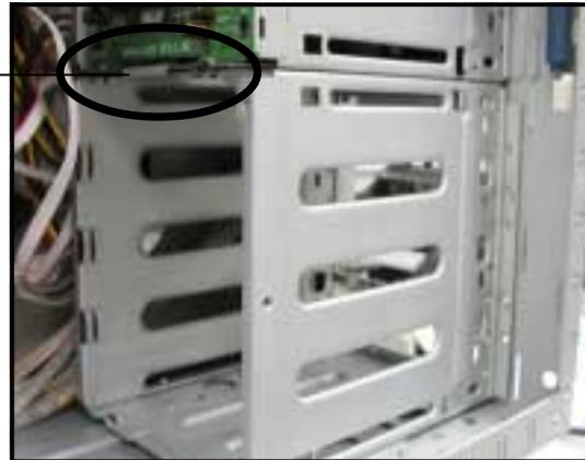
4. From the front side, secure the right side of the cage with two screws.
