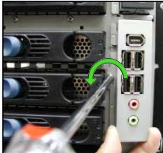
2. Carefully pull out the bracket until you see the cables connected to the I/O board.
