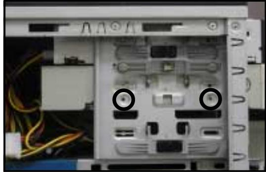
8. Pull down the bar lock and insert the lock pegs to the drive/bay holes, then push the drive lock to the right to secure the drive.
