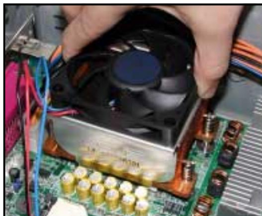
2. Use a Phillips screwdriver to tighten all four screws enough to secure the heatsink in place.
