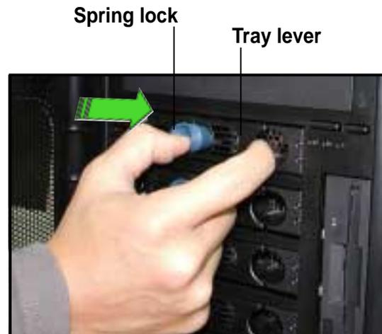
3. Firmly hold the tray lever and pull the drive tray out of the bay.
