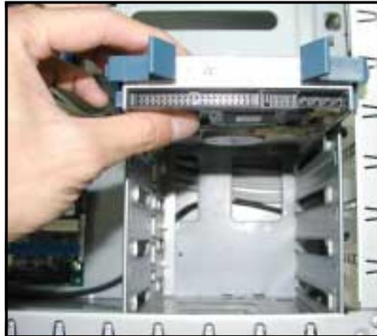
6. Connect the IDE and power cables to their corresponding connectors on the back of the drive.
