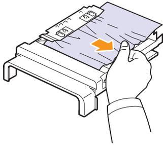
If the paper does not come out with the duplex unit, remove the paper from the bottom of the machine.
