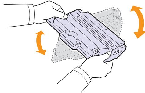
Thoroughly roll the cartridge to assure maximum copies per cartridge. Save the box and the plastic bag for shipping.
