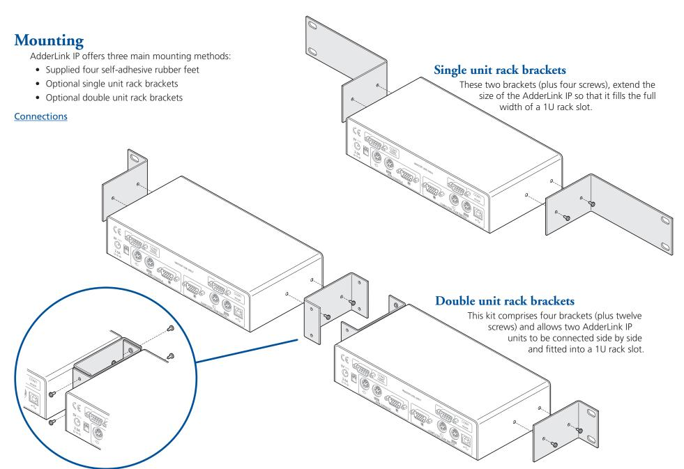
Installation of the AdderLink IP involves a number of basic connections to some or all of the following items:
