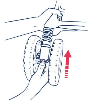
**CAUTION:** After wheel assembly is complete, pull on wheels to check that they are *locked* in place.
