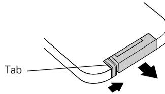
2. Remove the old battery and insert a CR2025 watch battery as shown.
