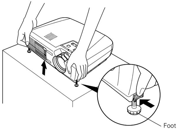
2. Once the image is positioned where you want it, release the levers to lock the feet in position.
