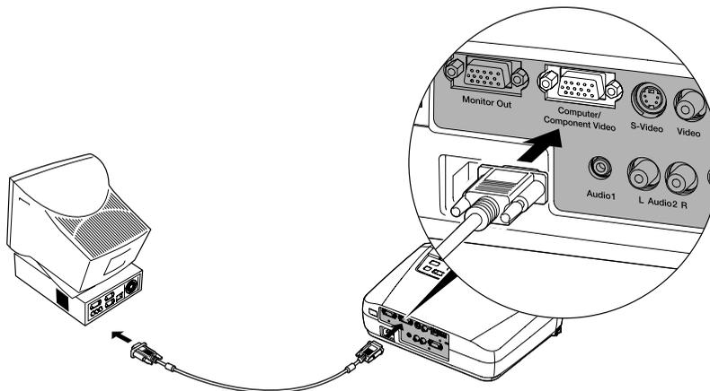
4. Connect the other end of the computer cable to the computer's video port.
