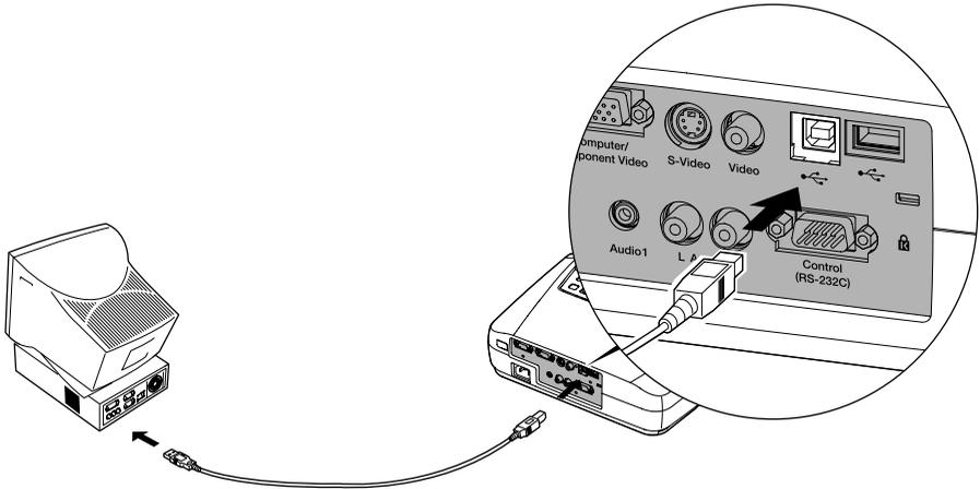
2. Disconnect your mouse from the USB port on the back of your computer and replace it with the other end of the cable. (Your computer's mouse will be disabled.)
