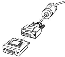
Replace the cover and connect the adapter to the free end of the computer video cable. Then plug the cable (with the adapter) into the video port on your Macintosh.
