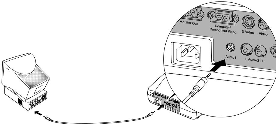
2. Connect the other end of the audio cable to the speaker or audio out port on the computer's sound card.
