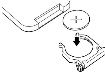
3. Slide the battery tray back into the remote until it clicks into place.
