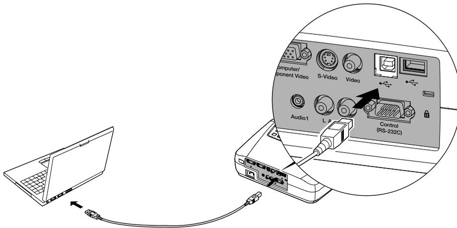
2. Connect the other end of the cable to the external mouse port or USB port on your laptop, as shown.
