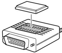
To use the adapter, remove its cover as shown and set its DIP switches according to the resolution you want to use, such as 16-inch mode. See your Macintosh documentation for instructions.
