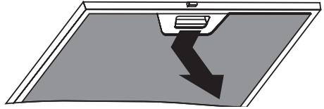
The metal grease filters should be washed, by hand, in mild soapy water or in a dishwasher. Allow to dry completely before replacing.
