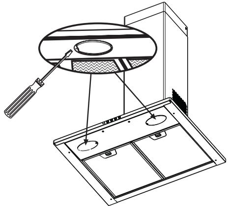
If the light bulb fails to function check that the bulb is fully screwed into the holder. If bulb failure has occurred then it should be replaced with a 220-240 Volt 40W clear globe shaped bulb with a small E14 screw thread.
