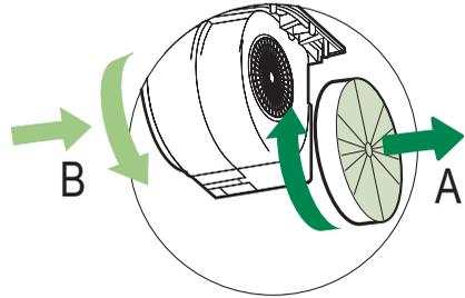
**⚠** This appliance can be a possible fire hazard if the grease and charcoal filters are not cleaned and replaced as recommended.
