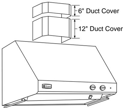
Decorative duct covers are available in 6" and 12" heights. Duct covers may be stacked, in various combinations, to conceal the ductwork running from the top of the hood to the ceiling.
