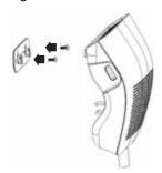
3 Mount the receiver onto the mounting bracket by sliding the slots on the bottom of the receiver downward onto the tabs on the bracket.
