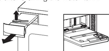
To drain the water tank:
