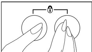
In order to activate the childproof lock, press the “Start/Pause/Cancel” and “Low temperature” buttons simultaneously for 3 seconds.
