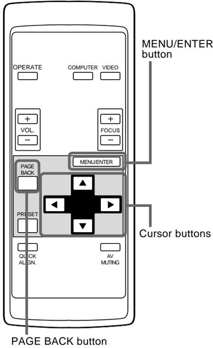
Adjust the position of the screen if it is displaced.
