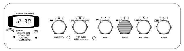
Push in and turn the control knob in either direction to vary the heat setting. The highest number represents the hottest setting and the lowest the coolest setting. Choose a setting appropriate to the quantity and type of food to be cooked.
