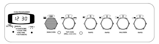
Push in and turn the main oven temperature control to the required setting.
