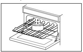
DO NOT place dishes or baking trays directly onto the oven base as it becomes very hot and damage may occur.
