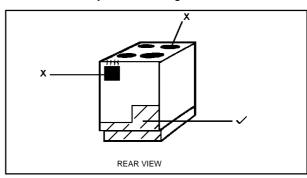
To move the cooker, open the main oven door, and lift the cooker by holding inside the top of the compartment.
