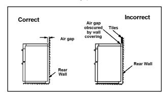
**Note:** Vapours from the oven vents may in time cause discolouration of wallcoverings behind the cooker. For ease of cleaning it may be preferable to tile behind the cooker.
