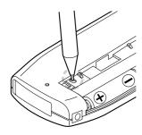
If the display or the recorder acts strangely, lightly press the reset button in the battery compartment with the tip of a ballpoint pen or a similar object.
