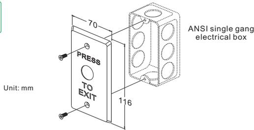
This series of request to exit can be mounted directly in ANSI electrical box (Flush mount)
