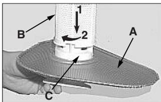
The entire filter assembly should be cleaned thoroughly once a month: cup C + semi-circular filter A + cylindrical filter B. Rotate filter "B" anticlockwise to remove it.
