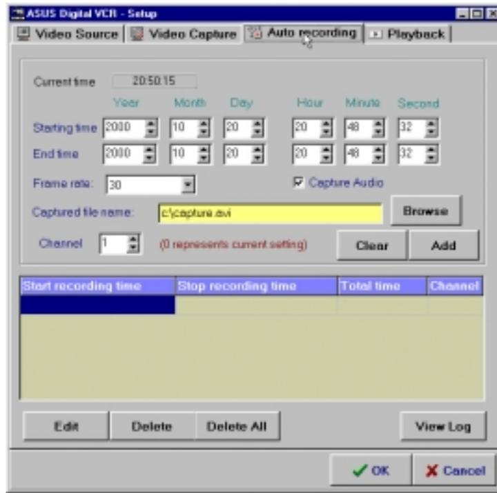
**Auto recording** includes the **Current time** (Hour:Minute:Second), **Start Time** (Year | Month | Day | Hour | Minute | Second), **End Time** (Year | Month | Day | Hour | Minute | Second), **Frame Rate**, **Channel**, and options to **Capture Audio** to the recording, **View Log** (of auto recorded events), and to **Delete** one or **Delete All** the pre-recording settings.
