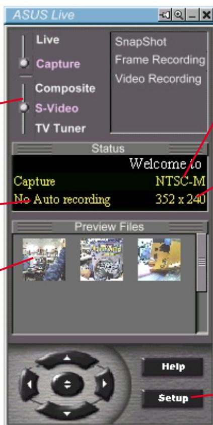
Click here to change the video standard (NTSC-M, NTSC-N, NTSC-4.43, PAL-BGHI, PAL-4.43, PAL-M, PAL-N or SECAM)
