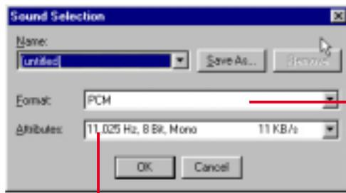
(PCM, which means Pulse Coded Modulation or uncompressed audio data, is currently the only available selection)
