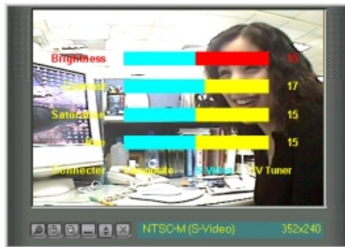
Use your mouse/pointing device or the UP and DOWN arrow keys on your keyboard to select options (*Brightness, Contrast, Saturation, Hue, Connector*) and then the LEFT (select to the left or to decrease) or RIGHT (select to the right or to increase) arrow keys to change an option. You may also use your mouse/pointing device to change an option by clicking the appropriate item or slider.
