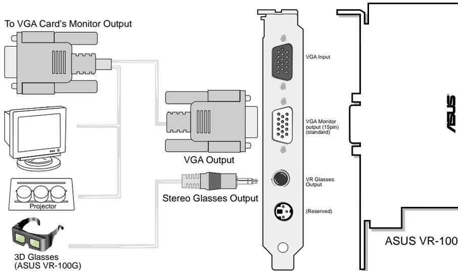
When using a Y-type cable, you do not need to connect the VGA Input of the VR-100 to your VGA card's monitor output (see diagram above).
