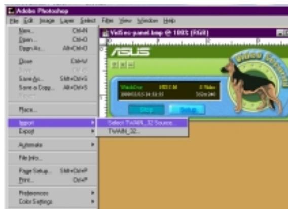
**NOTE:** You do not need to repeat this step for subsequent uses of the ASUS TWAIN module. If more than one TWAIN device is installed in your system and you want to switch devices, use **Select TWAIN\_32 Source** command.
