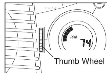
Rotate the thumb wheel on the right side of the fan to pivot the fan to the desired angle.
