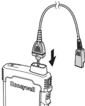
3. Attach the quick disconnect end of the headset adapter cable to the headset's cable.
