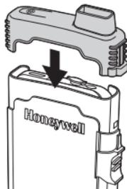
10. Slide the lock closed to secure the end cap.
