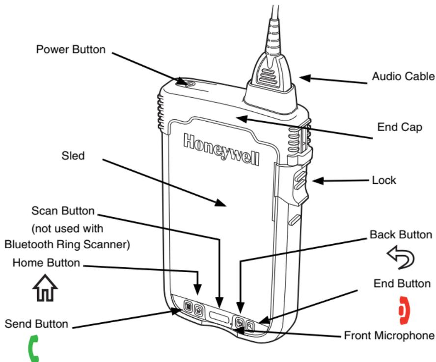
The sled encases the Dolphin 70e Black including the touch panel and helps protect the terminal from impacts.
