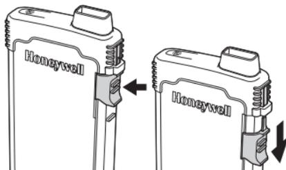
3. Push up on the right side of the end cap. Do not attempt to remove the end cap without opening the lock first!
