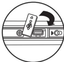
5. Press until the door is flush with the side of the terminal.
