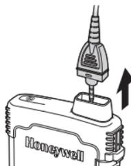
2. Slide the lock down to release the end cap.
