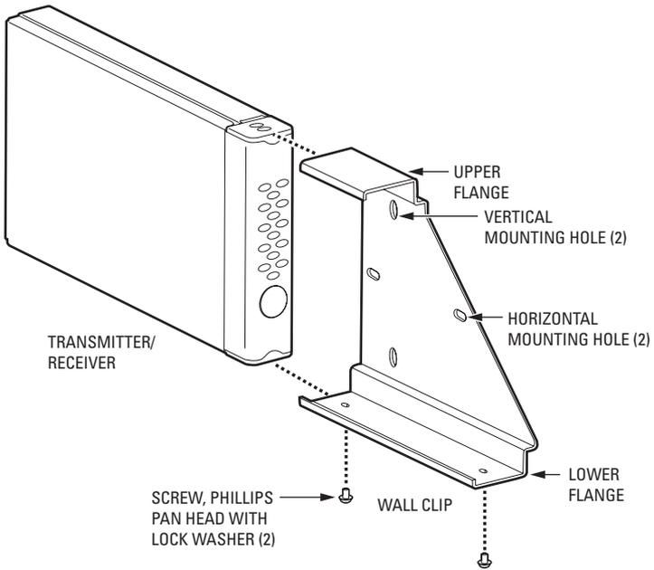
**Figure 5.** Mounting the FT8304 Transmitter/FR8304 Receiver Using the Wall Clip
