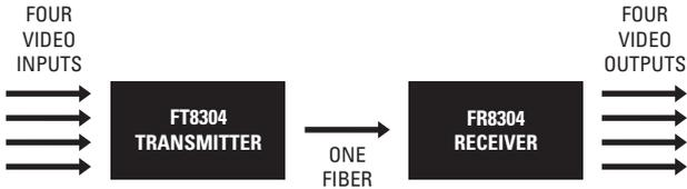
**Figure 1.** Four-Channel Video FT8304 Transmitter and FR8304 Receiver
